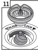
11 Push upper burr firmly into position
